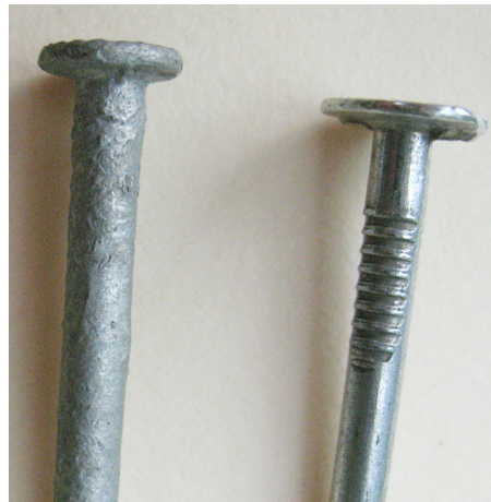
The nail on the left is double hot-dipped galvanized. The nail on the right is electroplated.
