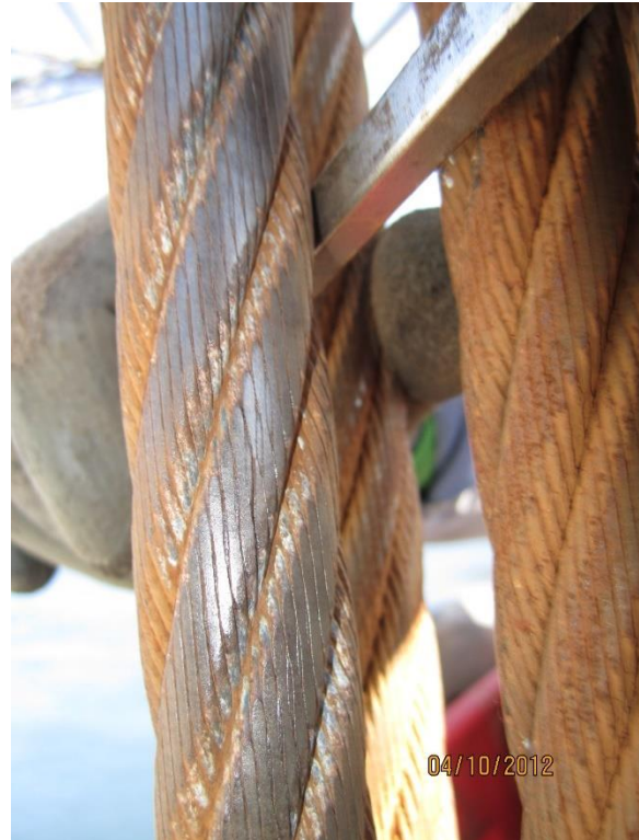
Figure 1: Heavy wear on the sides of the ropes that has progressed through the outer layer of wires. The ropes were only in service for approximately 10 years.
